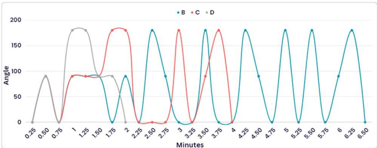
Figure 9. Angle-Time Graph of the Servo Motor
