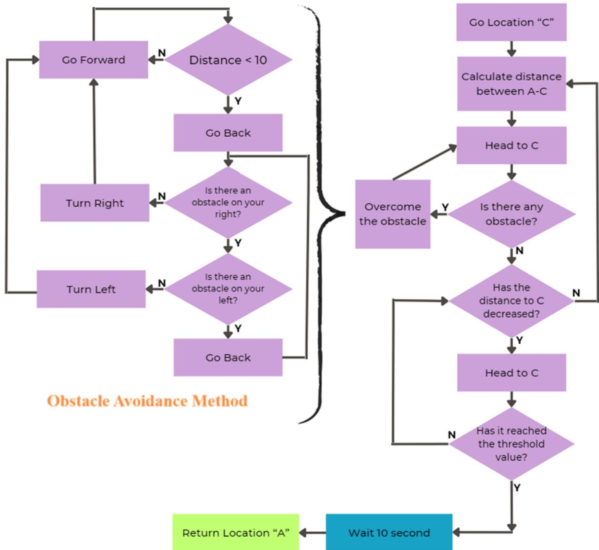
Figure 5. Flow Diagram of the Direction Detection Algorithm
