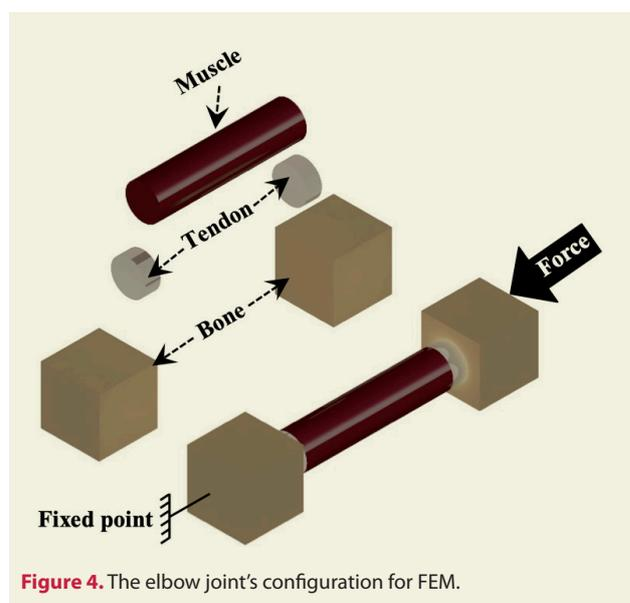
**Figure 4.** The elbow joint's configuration for FEM.
