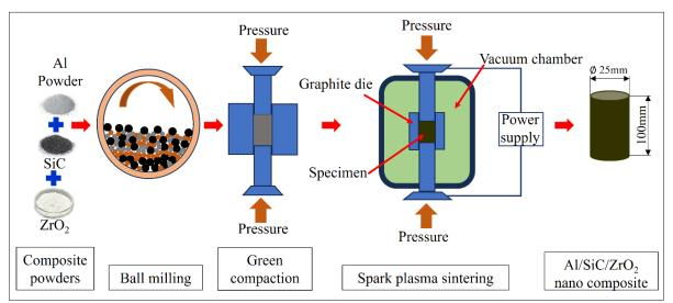
Figure 2. Schematic diagram of spark plasma sintering (SPS) process
