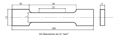
Figure 4. ASTM E-8-04 standard tensile test specimen
