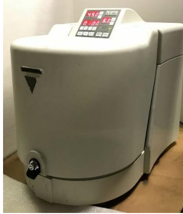
Figure 1. Shows planetary mono mill pulverisette 6 classic line
