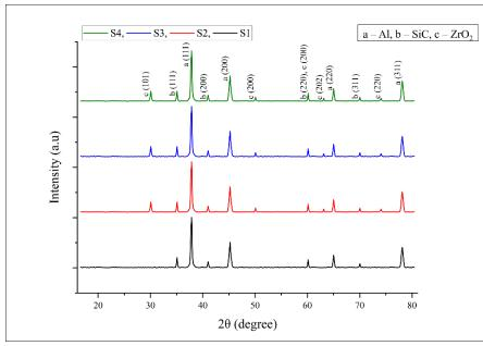
Figure 5. Shows the hybrid Al/SiC/ZrO<sub>2</sub> composite of XRD patterns
