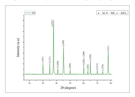
Figure 6. XRD pattern for sample S4
