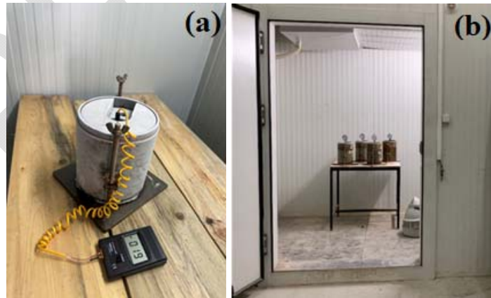
Figure 5 - Freeze-thaw test a) Image showing temperature measurements in control samples using a thermocouple b) images of CBR samples with a dial gauge inside the chamber.
