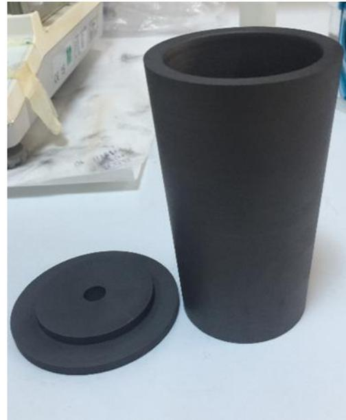
Figure 1. Graphite crucibles used in the experiments
