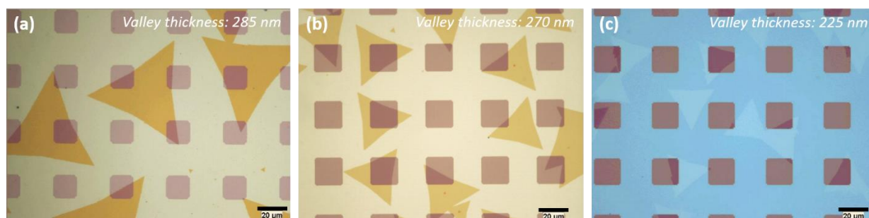
Figure 2. Monolayer MoS 2 flakes on patterned surfaces with valley thicknesses of (a) 285 nm (15 nm depth), (b) 270 nm (30 nm depth), and (c) 225 nm (75 nm depth)
