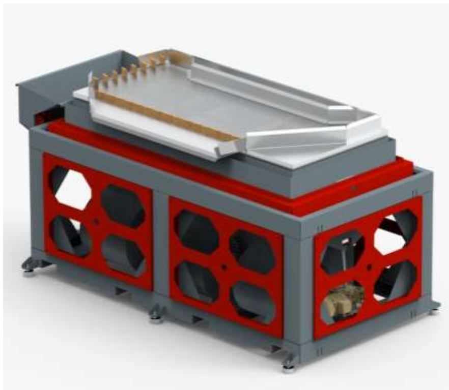
Figure 6. Rendered image of the gravity separator design for the recovery of two different metal groups.
