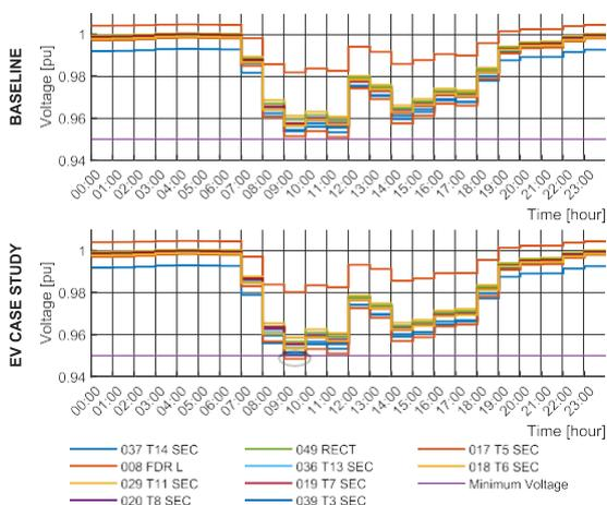
**Fig. 4.** Quasi-dynamic results: time-voltage profiles.
