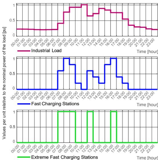
**Fig. 2.** Time-load profiles for quasi-dynamic simulations.
