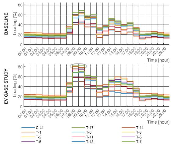
**Fig. 3.** Quasi-dynamic results: time-loading profiles.
