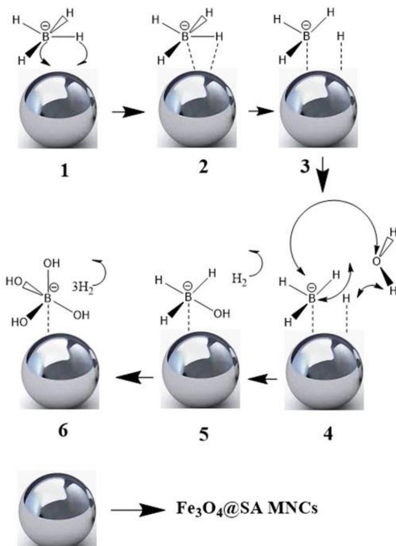
**Figure 10:** A possible mechanism of  $\text{NaBH}_4$  hydrolysis catalyzed by  $\text{Fe}_3\text{O}_4$ @SA MNCs.
