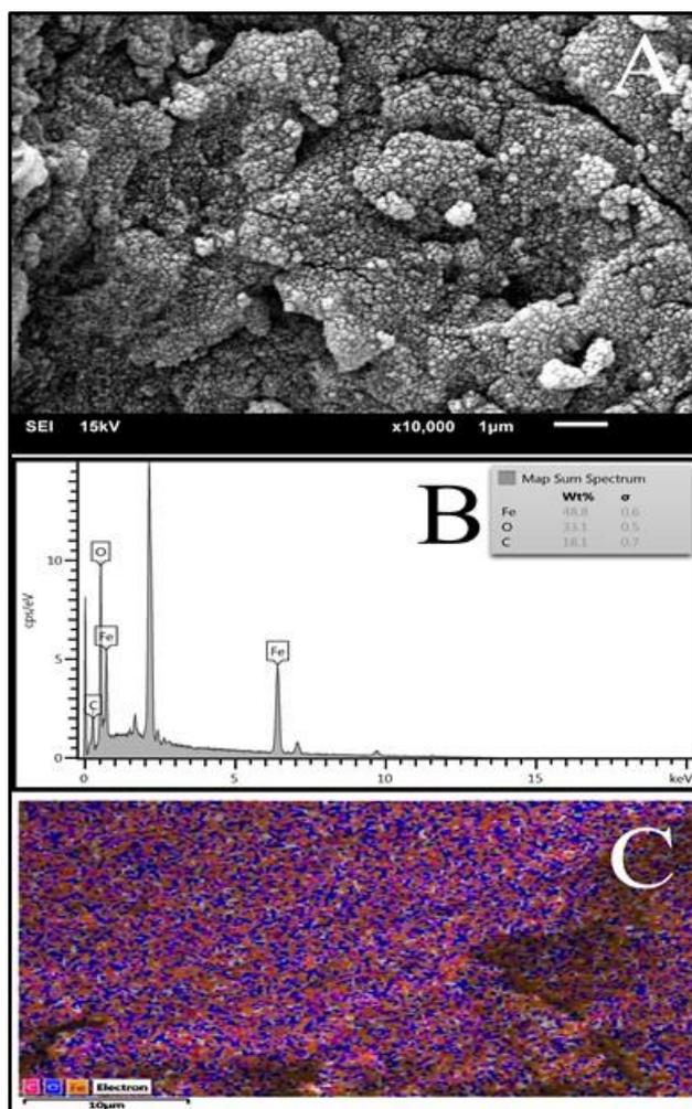
Figure 5: Fe<sub>3</sub>O<sub>4</sub>@SA MNCs A) SEM images, B) SEM-EDS graph, C) SEM-EDS-map graph.
