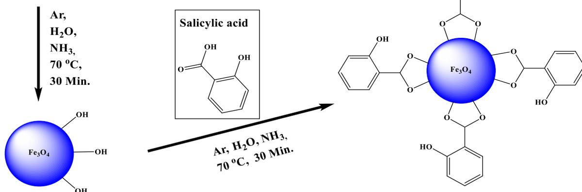
**Figure 1.** The synthesis scheme of Fe<sub>3</sub>O<sub>4</sub>@SA MNCs.
