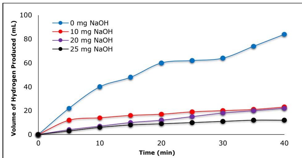
**Figure 6:** Effect on hydrogen volume in NaBH<sub>4</sub> hydrolysis of NaOH (Reaction conditions: 50 mg Fe<sub>3</sub>O<sub>4</sub>@SA MNCs, 100 mg NaBH<sub>4</sub>, 0, 10, 20 and 25 mg NaOH and 25 °C).
