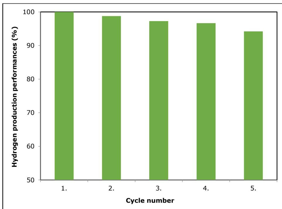
**Figure 9:** The reusability of Fe<sub>3</sub>O<sub>4</sub>@SA MNCs for hydrolysis of NaBH<sub>4</sub> at 25 °C.
