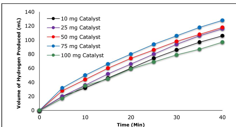
**Figure 8:** Effect on hydrogen volume by hydrolysis of NaBH<sub>4</sub> of Fe<sub>3</sub>O<sub>4</sub>@SA MNCs (Reaction conditions: 10, 25, 50, 75, and 100 mg Fe<sub>3</sub>O<sub>4</sub>@SA MNCs, 150 mg NaBH<sub>4</sub> and 25 °C).
