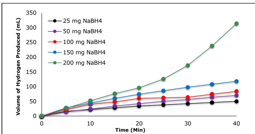
**Figure 7:** Effect on hydrogen volume of NaBH<sub>4</sub> using Fe<sub>3</sub>O<sub>4</sub>@SA MNCs (Reaction conditions: 50 mg nano-catalyst, 25, 50, 100, 150 and 200 mg NaBH<sub>4</sub> and 25 °C).
