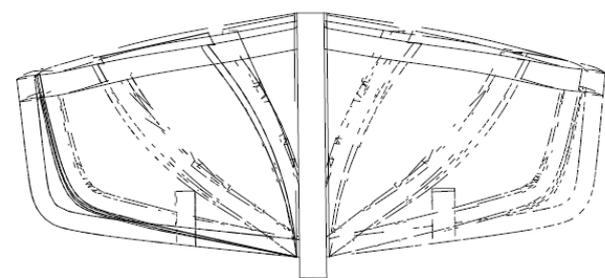
**Figure 7.** Front view of the structure and framing system of Perahu Bedar
