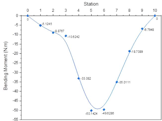
**Figure 11.** Bending moment along the Perahu Bedar
