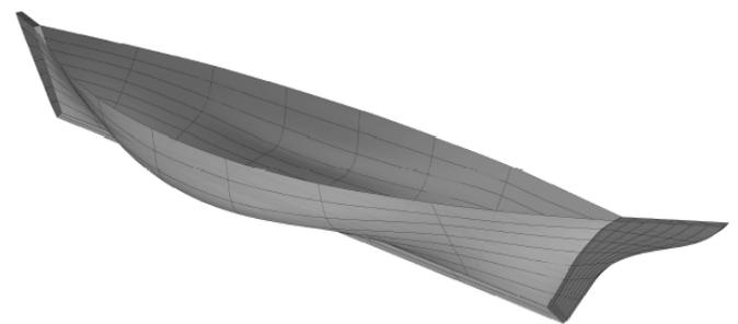
**Figure 3.** 3-D surface modelling of Perahu Bedar
