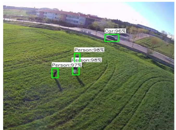
Figure 9. Object Detection using SSD MobileNetV2 model with Edge TPU
