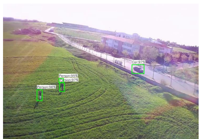
Figure 10. Human Detection using SSD MobileNetV2 model with Edge TPU
