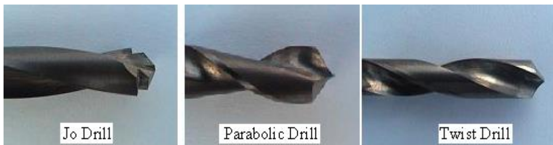
Figure 1. Drill point geometry [34]
