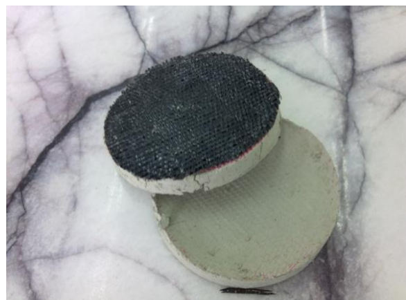
Figure 1. Consolidation test samples placed with geotextile (Dikmen, 2013)
