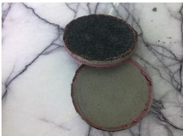
Figure 1. Consolidation test samples placed with geotextile (Dikmen, 2013)
