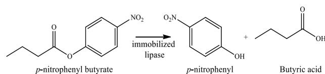
**Figure 1.** The catalytic reaction of *p*-nitrophenyl butyrate
