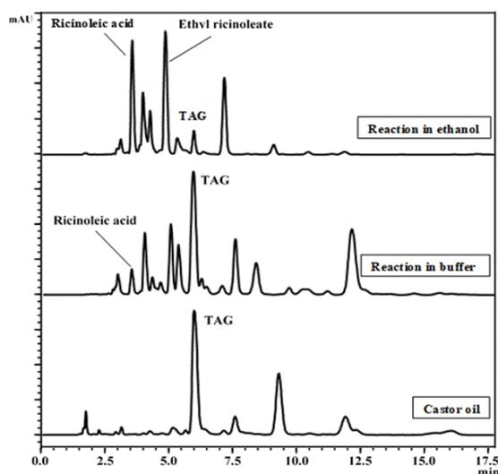
**Figure 3.** HPLC chromatograms of castor oil and products after hydrolysis/transesterification reactions. (72 h, 150 rpm, 2.5 mL lipase immobilized agarose beads, 1.0 g castor oil, 25 mL reaction volume)
