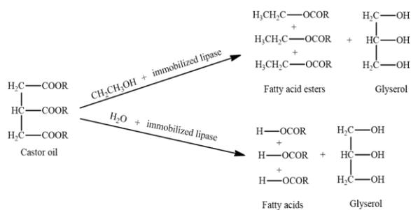
**Figure 5.** Hydrolysis and transesterification reactions of castor oil**Table 2.** The effect of castor oil amount on the hydrolysis/transesterification of castor oil with immobilized lipase
