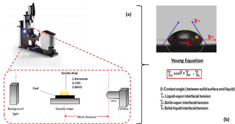
**Figure 4.** (a) The illustration of the contact angle goniometer (b) schematic representation of wetting statics in Young's equation for solid-liquid-vapor system.
