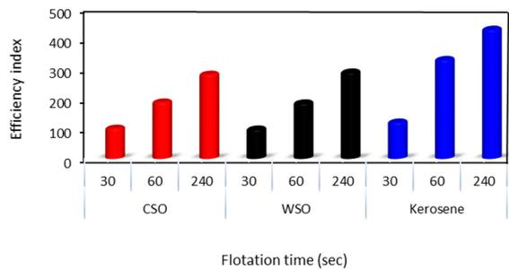
**Figure 8.** Flotation efficiency index (EI) at various collecting times with WSO, CSO, and kerosene.
