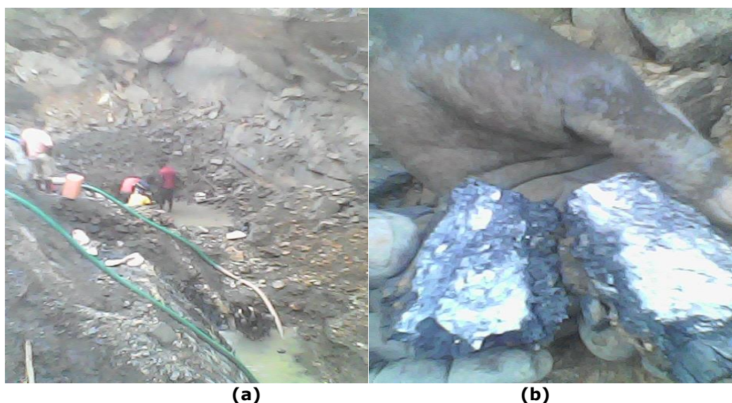
Figure 1: Pb–Zn Mine at Adudu Showing Mine Wastewater Discharged or pumped to Nearby Farmlands (a) and the Pb–Zn ore (b) being mined.
