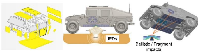
Fig. 1. Application on wheeled armored vehicles of sandwich panels with metal foam and cellular porous core [3].
