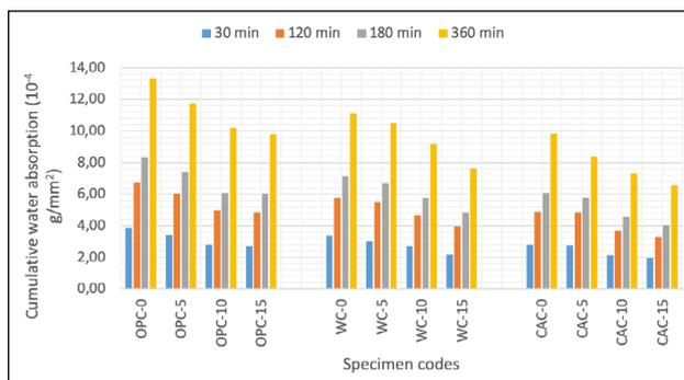
Figure 5. Cumulative capillary water absorption results of mixtures.
