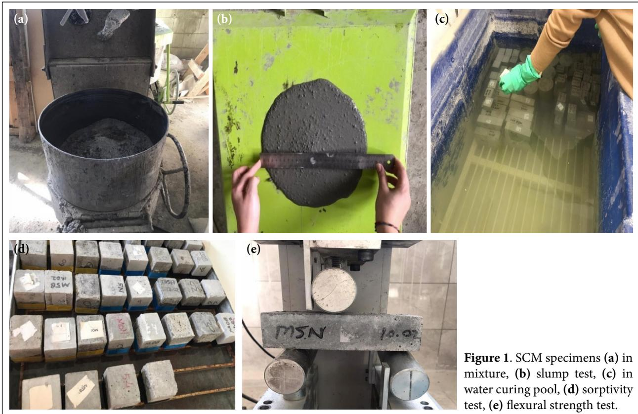
**Figure 1.** SCM specimens (a) in mixture, (b) slump test, (c) in water curing pool, (d) sorptivity test, (e) flexural strength test.
