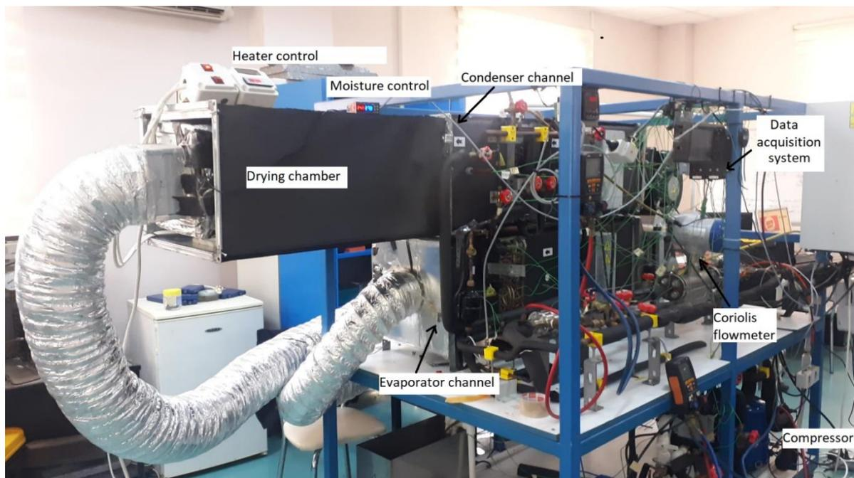
**Figure 1.** The heat pump drying system
