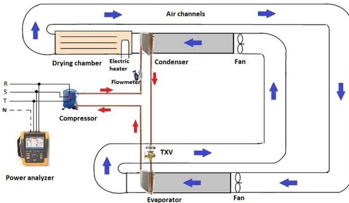
**Figure 2.** Paths followed by refrigerant flow and airflow in the HPD system
