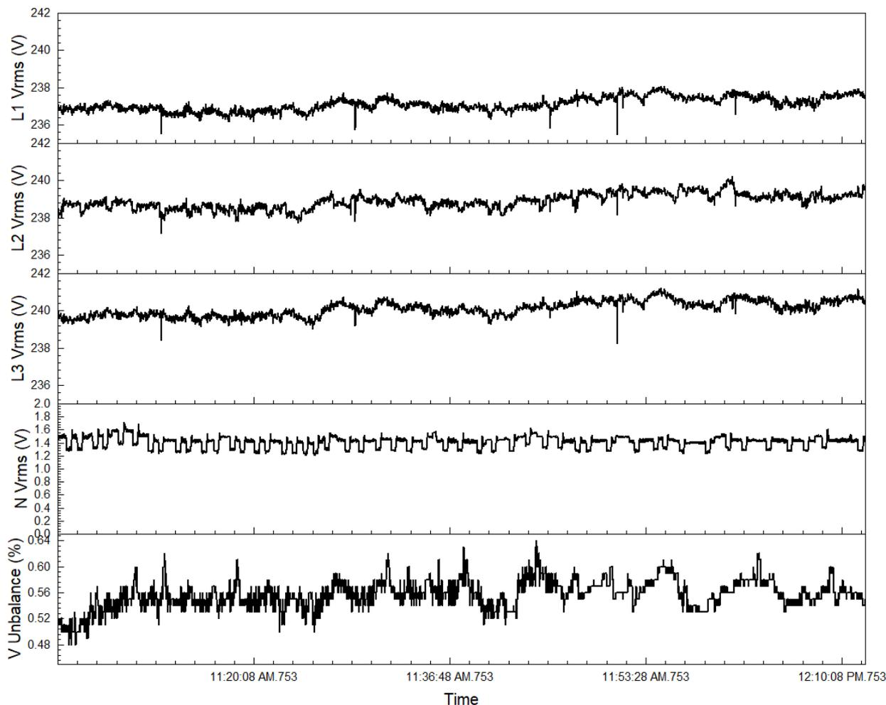
**Figure 7.** Time-dependent voltage values for all three phases and the neutral line, along with the voltage imbalance in the system.
