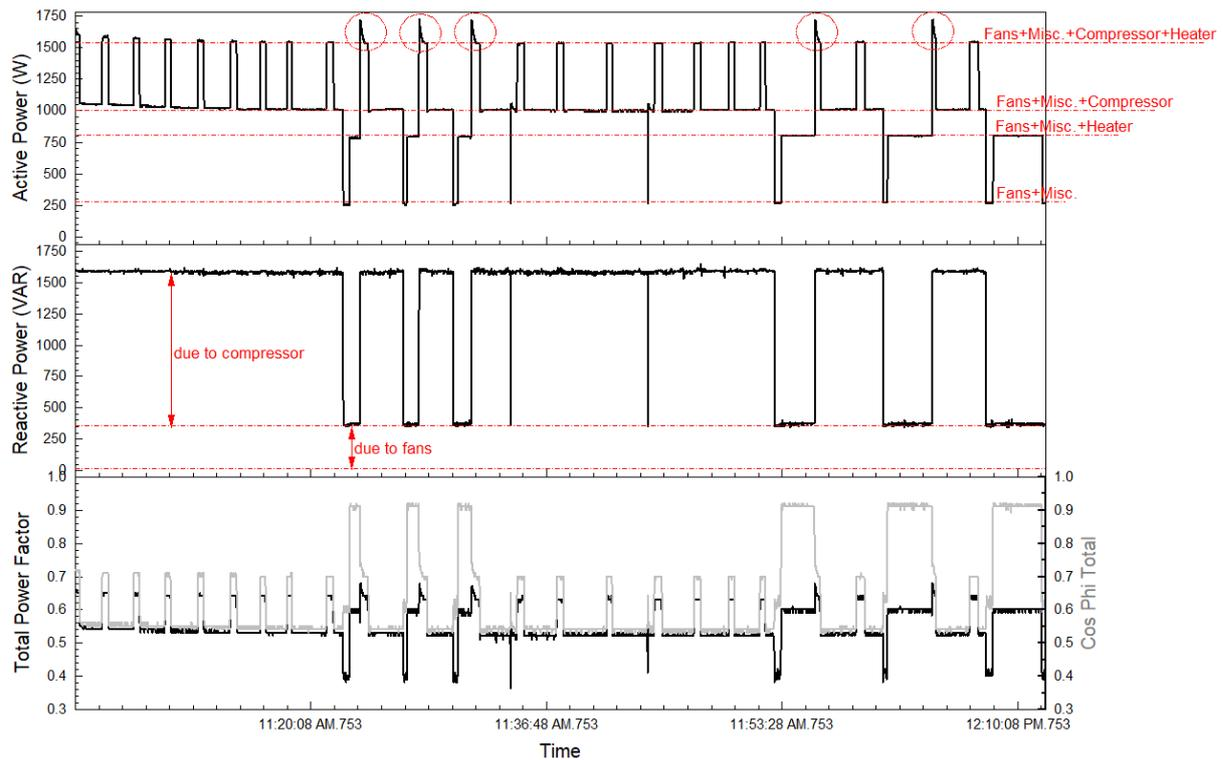
**Figure 4.** Active power, reactive power, total power factor, and displacement power factor values drawn by the HPD system.
