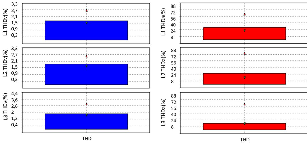
Figure 5. Histogram graph showing voltage and current harmonics for each phase.
