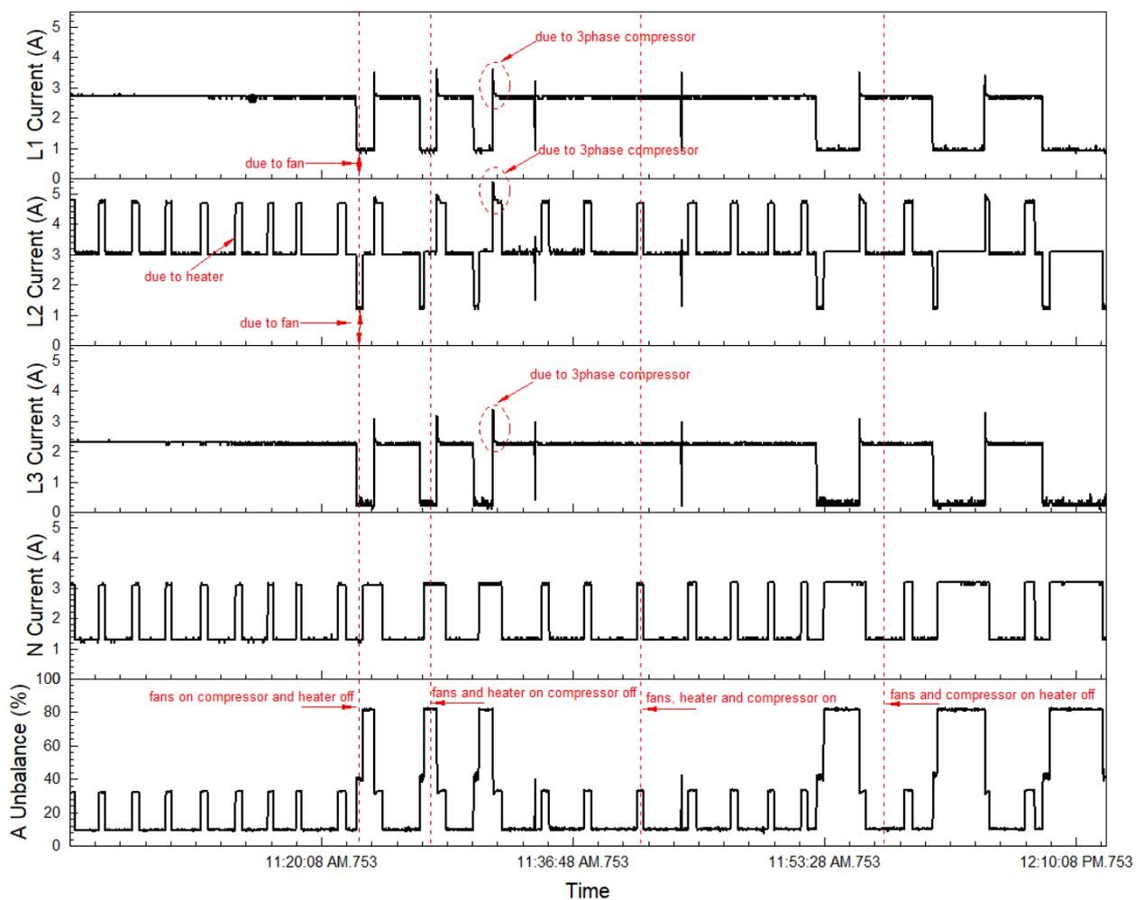
**Figure 8.** Time-dependent current for each of the three phases and the neutral line, along with the graph showing current imbalance in the system.
