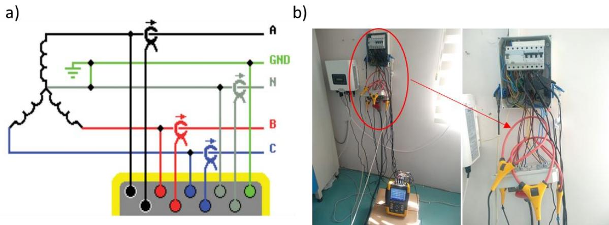
**Figure 3.** a) connection diagram of the probes to the three-phase system b) real image of the installation of the measurement setup into the system
