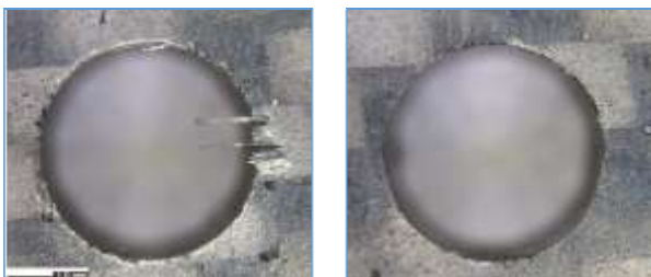
Figure 5. Delamination images for feed rate; a) Constant, b) Varying
