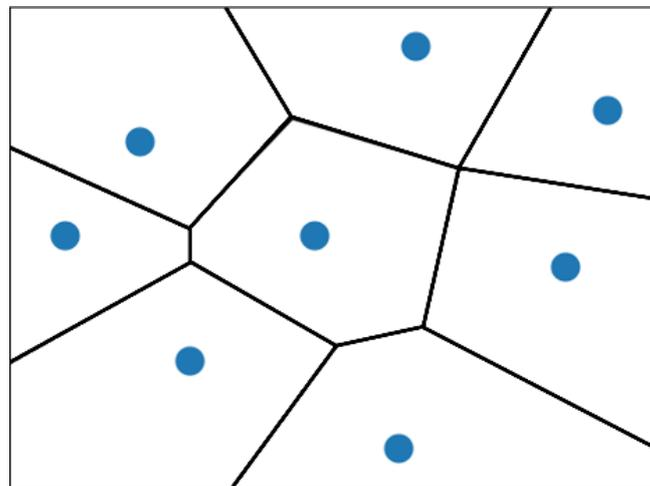
Figure 1. Voronoi diagram example for 8 points
