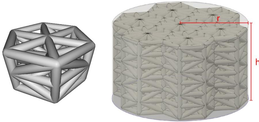
**Figure 2.** Circular pattern hexagonal lattice model
