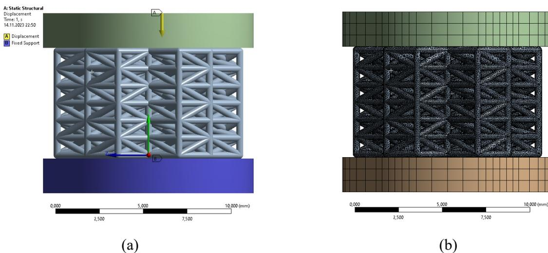
**Figure 4.** a) 3D FEA model b) FEM boundary conditions
