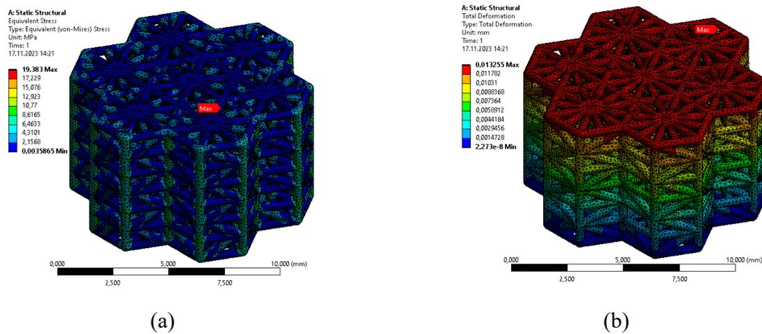
**Figure 5.** a) von Mises stress result b) Maximum displacement result
