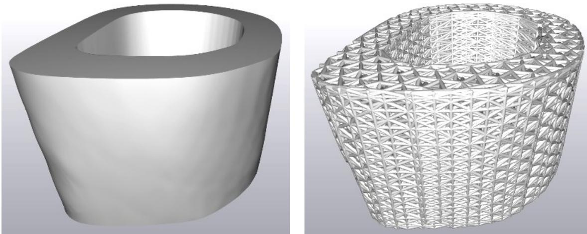
**Figure 3.** Hexagonal lattice model in the femur bone structure
