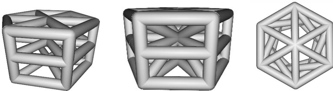
**Figure 1.** 3D model of hexagon strut-based lattice geometry
