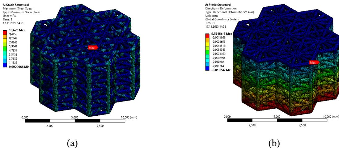
**Figure 6.** a) Maximum shear stress result b) Z-Directional deformation result
