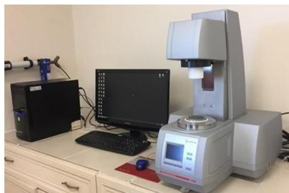
**Figure 2.** Anton Paar MCR 102 Rheometer.
