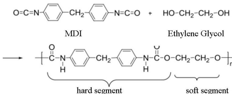
Figure 4. Chemical reaction between MDI and polyethylene glycol.
