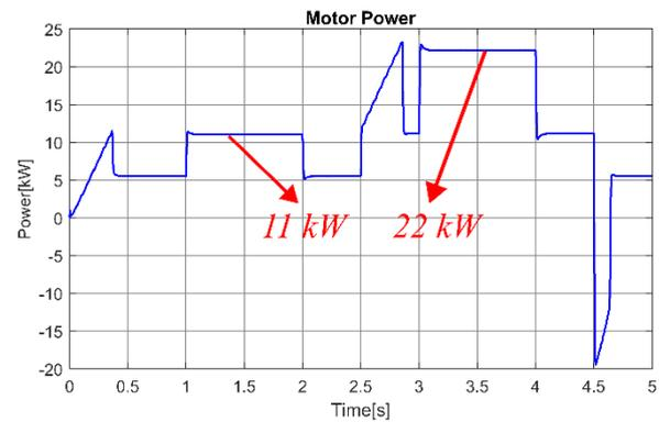
Fig. 14. Output power of the designed motor
