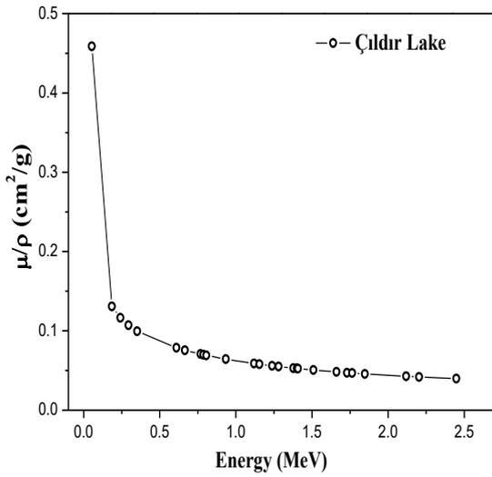
**Figure 5.** Variation of mass attenuation coefficients with energy for Çıldır Lake average value
