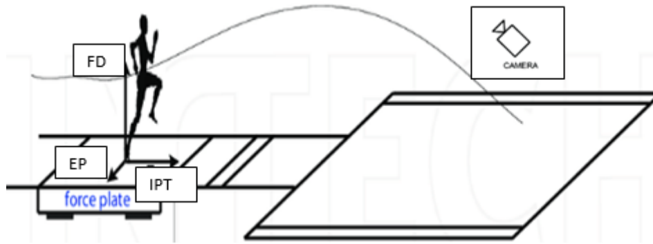
FD:Flight Distance, EP: Explosive Power, IPT: Instant Push Time
