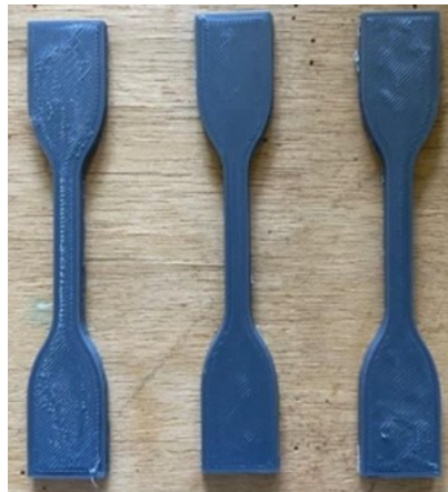
Figure 4: Samples of printed specimens for various annealing times: 20, 40 and 60 min (from left to right)
