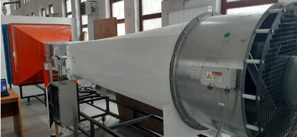
Fig.1. Subsonic Wind Tunnel
