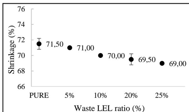
**Figure 14.** Graphical representation of shrinkage values of LEL films
