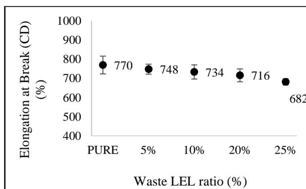
**Figure 8.** Graphical representation of CD elongation at break values of LEL films
