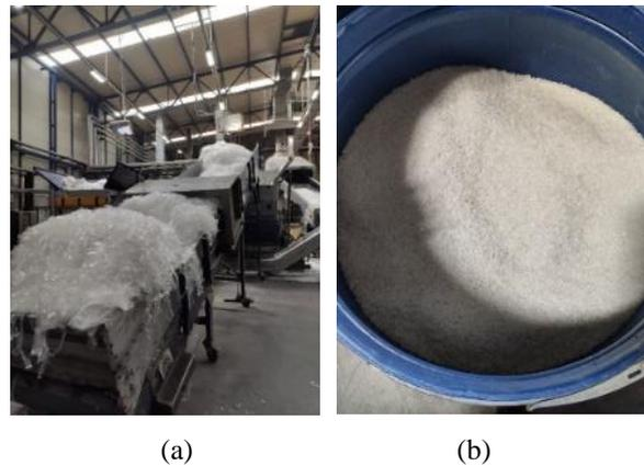
**Figure 1.** Granules produced from single screw extruder
