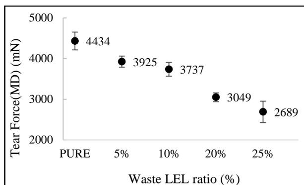
**Figure 9.** Graphical representation of MD tearing force values of LEL films
