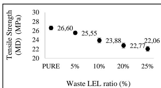
**Figure 3.** Graphical representation of MD tensile strength values of LEL films
