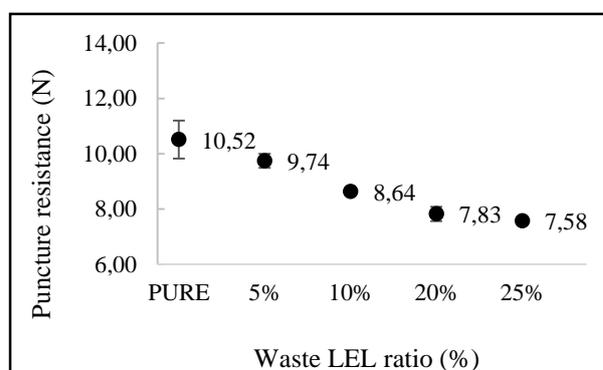
**Figure 11.** Graphical representation of puncture force values of LEL films
