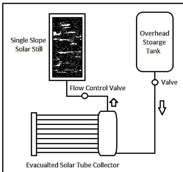
**Figure 9.** Schematic diagram of the solar still coupled with an evacuated tube solar collector.
