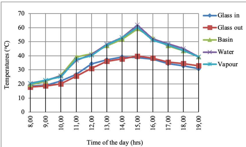
Figure 14. Relationship between solar still temperature with respect to time of the day.
