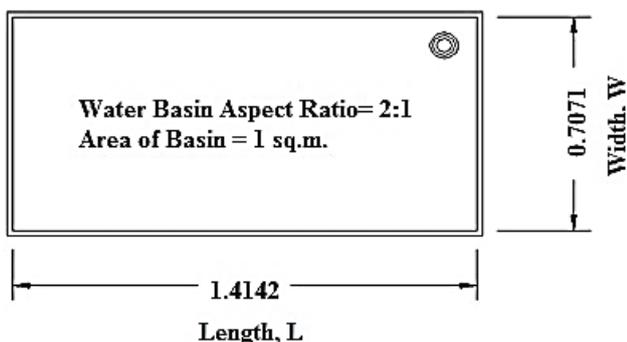
Figure 1. Basin area of solar still with aspect ratio 2:1.
