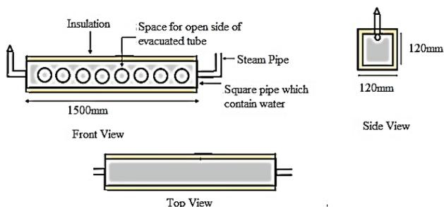
**Figure 8.** Cross Sections of Header.
