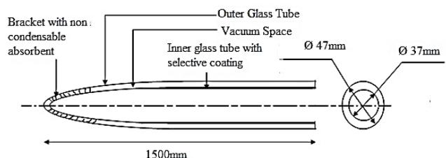
Figure 7. Cross section of borosilicate evacuated tubes.
