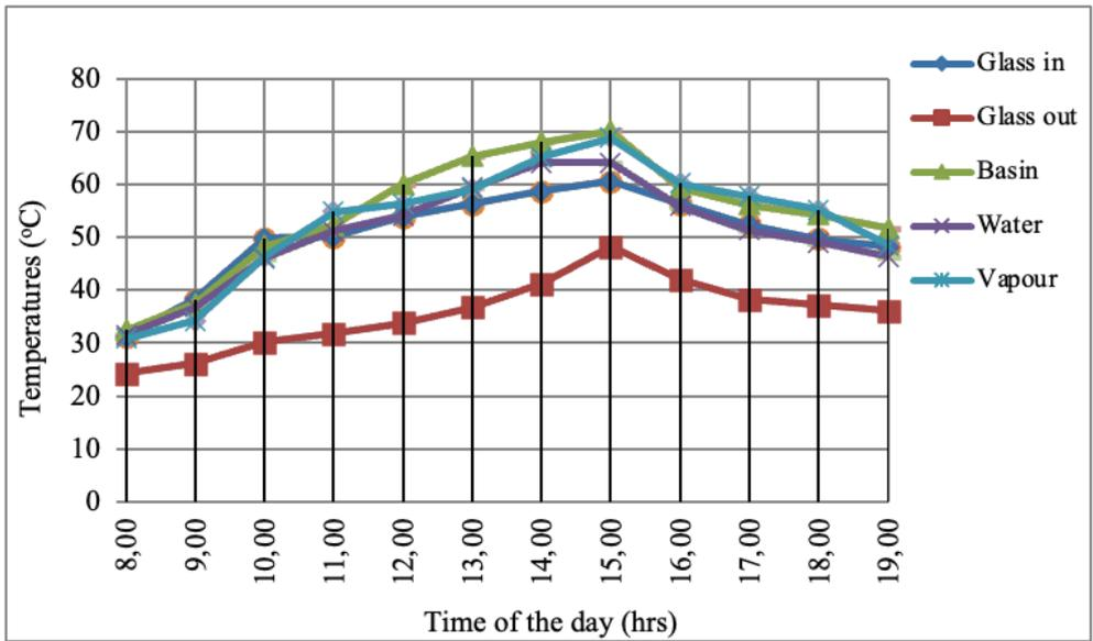
Figure 18. Relationship between solar still temperature with respect to time of the day.
