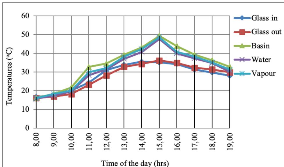
Figure 11. Relationship between solar still temperature with respect to time of the day.
