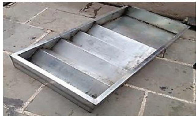
Figure 2. Stepped absorber plate.
