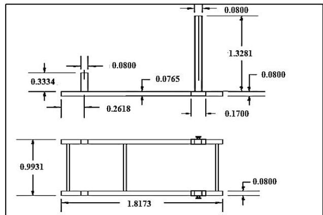
Figure 3. Stand used for mounting the solar still.
