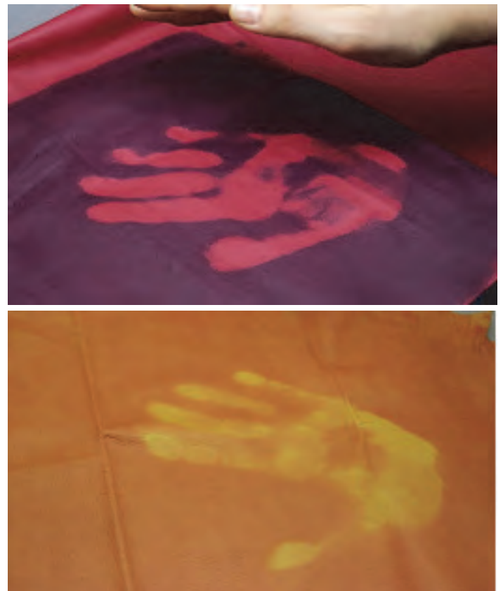
Figure 1. The display of cold activated (above) and touch activated thermochromic leathers (below)
