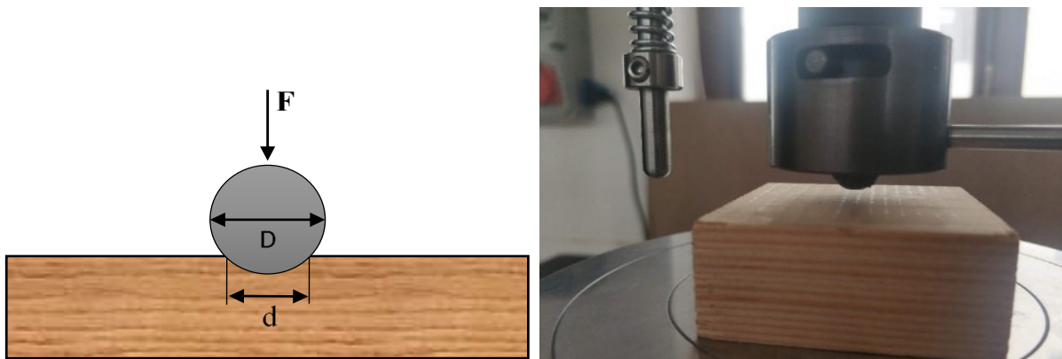
Figure 4. Brinell Hardness test and its application method
