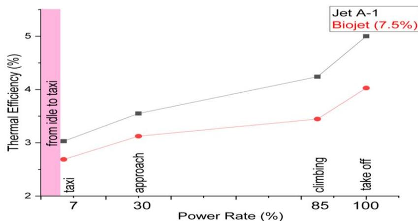
**Figure 2.** The effect of biojet blend on thermal efficiency
