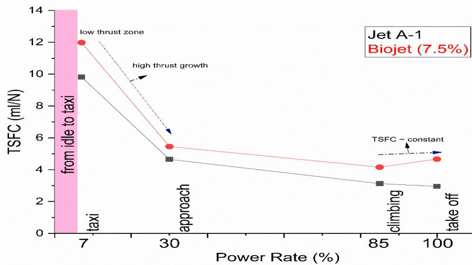
Figure 4. The effect of bio jet at different power ratios on TSFC
