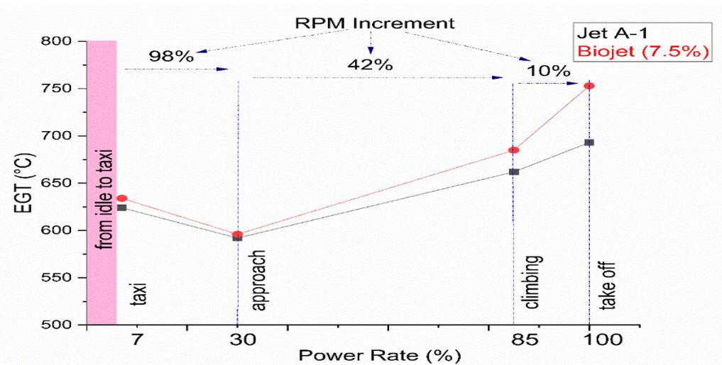
Figure 5. The effect of bio jet at different power ratios on exhaust gas temperature
