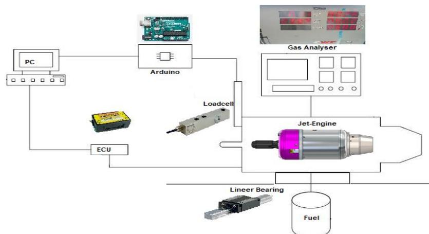
**Figure 1.** Schematic representation of the experiment set
