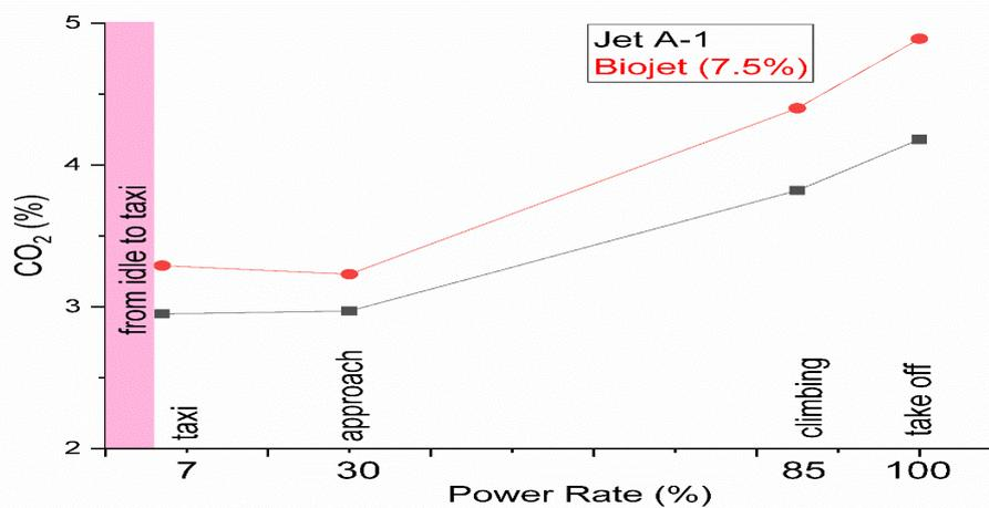
Figure 6. The effect of bio jet at different power ratios on CO<sub>2</sub> emission
