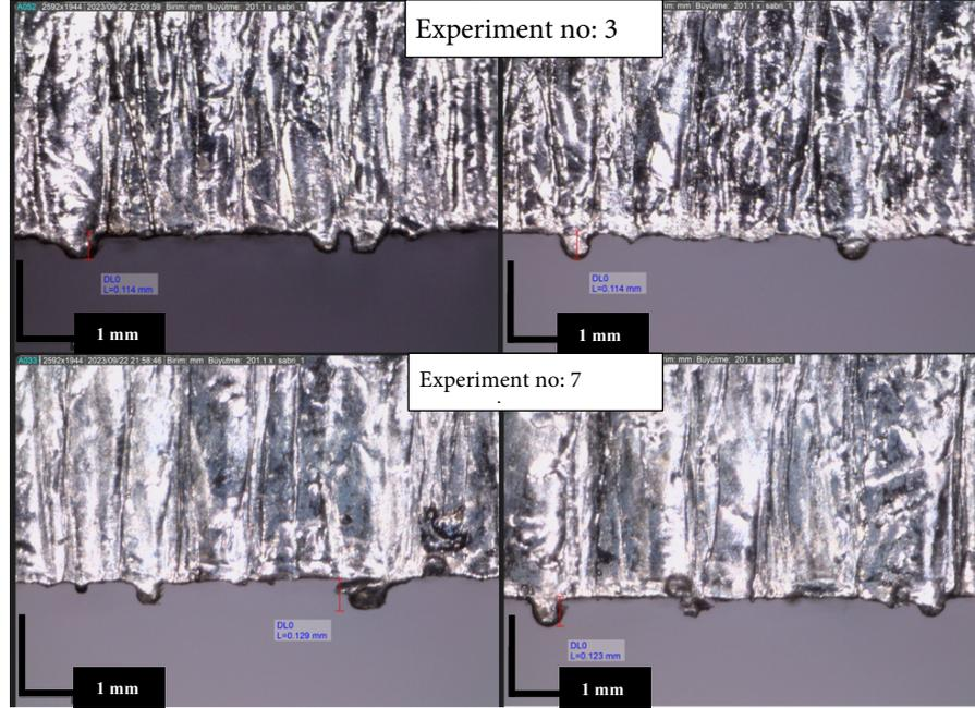
Figure 5. Burr formations in the bottom kerf width
