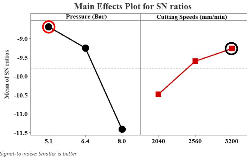
Figure 7. Signal/noise ratios for pressure and cutting speed.
