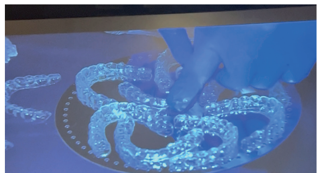
Figure 4: Graphy Shape Memory Clear Aligner curing stage
