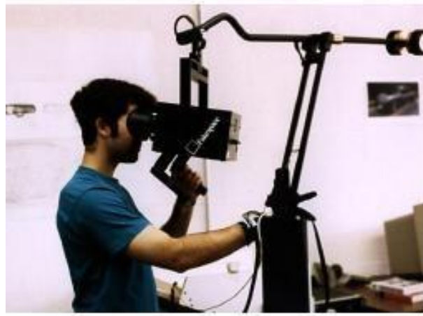
Resim 4. BOOM (Binocular Omni-Orientation Monitor).
