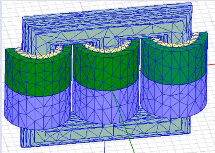
Figure 1. ANSYS model of the transformer
