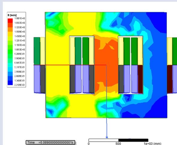
Figure 2. Instantaneous magnetic flux variation at THD=0
