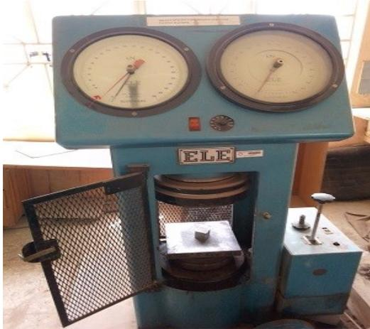
Fig. 3. Compressive testing machine
