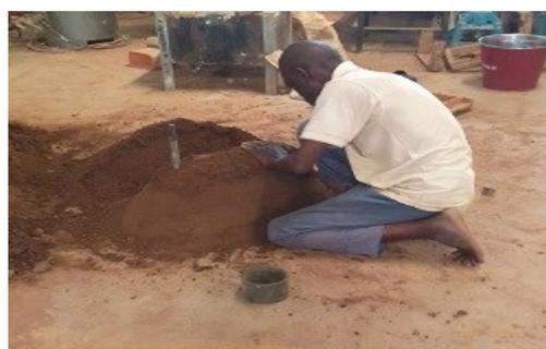
**Fig. 2.** Making of moulds from laterite soil
