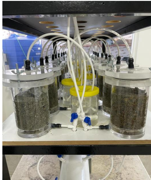
Figure 5. Kinetic test setup view
