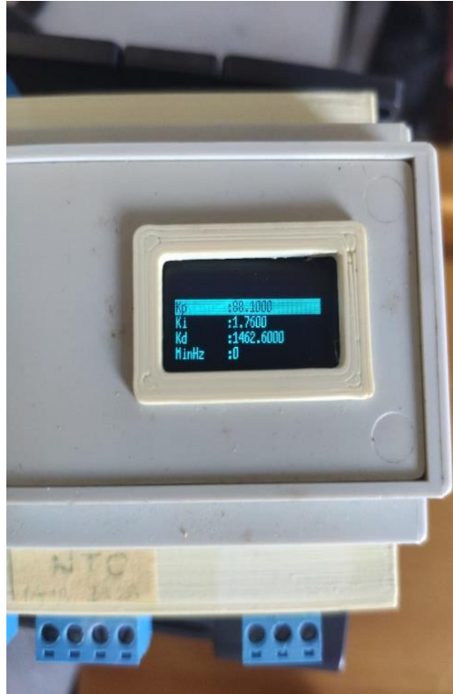
Figure 7. PID parameters determined by self-tune
