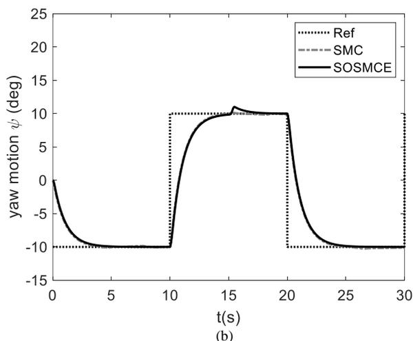
Figure 3. Tracking reference a) pitch motion, b) yaw motion
