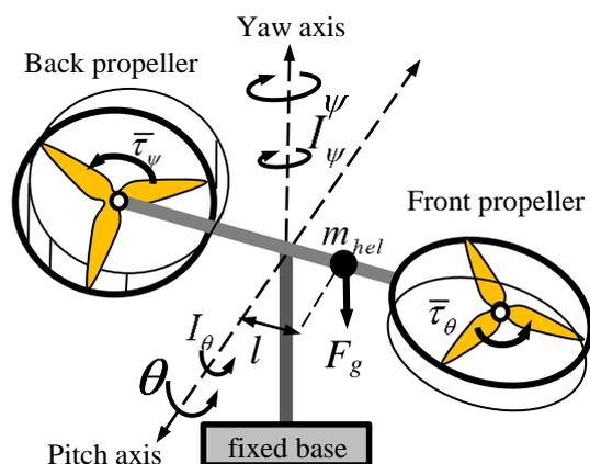
Figure 1. The physical of the twin rotor
