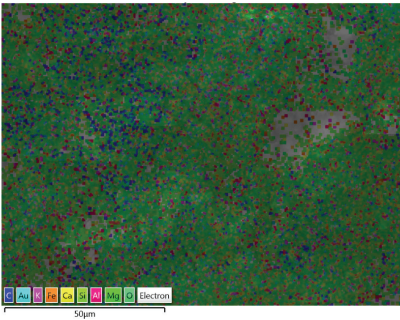
Figure 6 - EDS layered image of D2 diatomite
