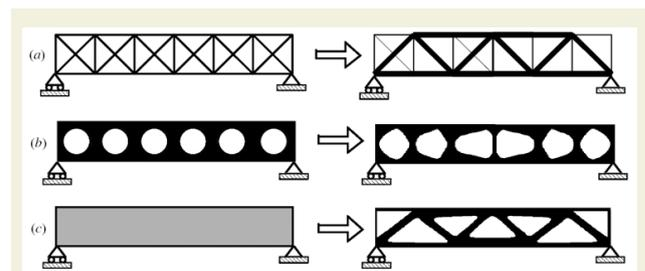
Figure 2. Structural Optimization, a) Sizing optimisation, b) Shape and c) Topology optimisation[10].
