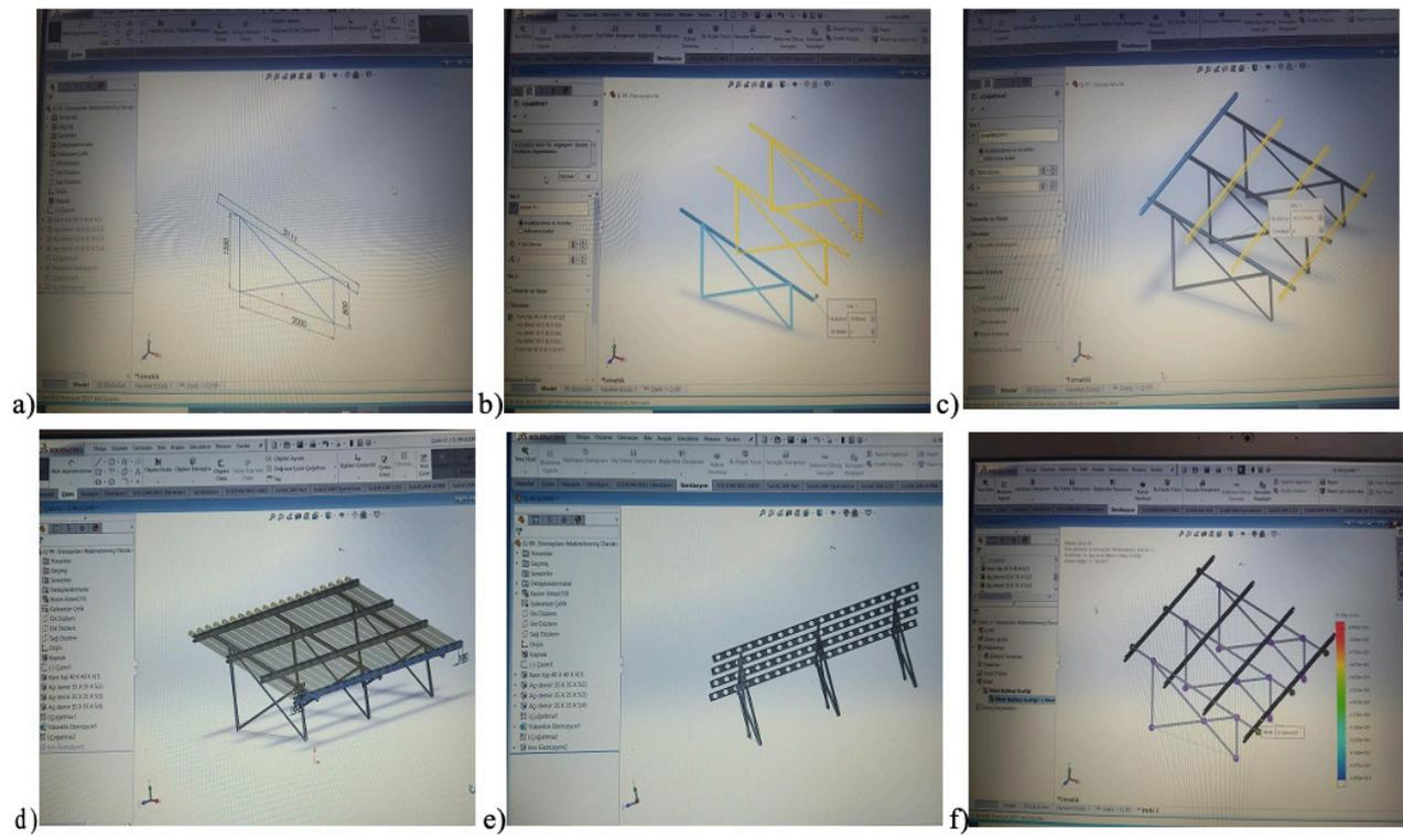
**Figure 9.** Selected sample part Selected sample part; a) Drawing the bottom profiles, b) Creating the bottom profiles, c) Placing the C profiles, d) Determination of the areas to be emptied from C profiles, e) Emptied version of the design, f) Creating the mesh structure of the design.
