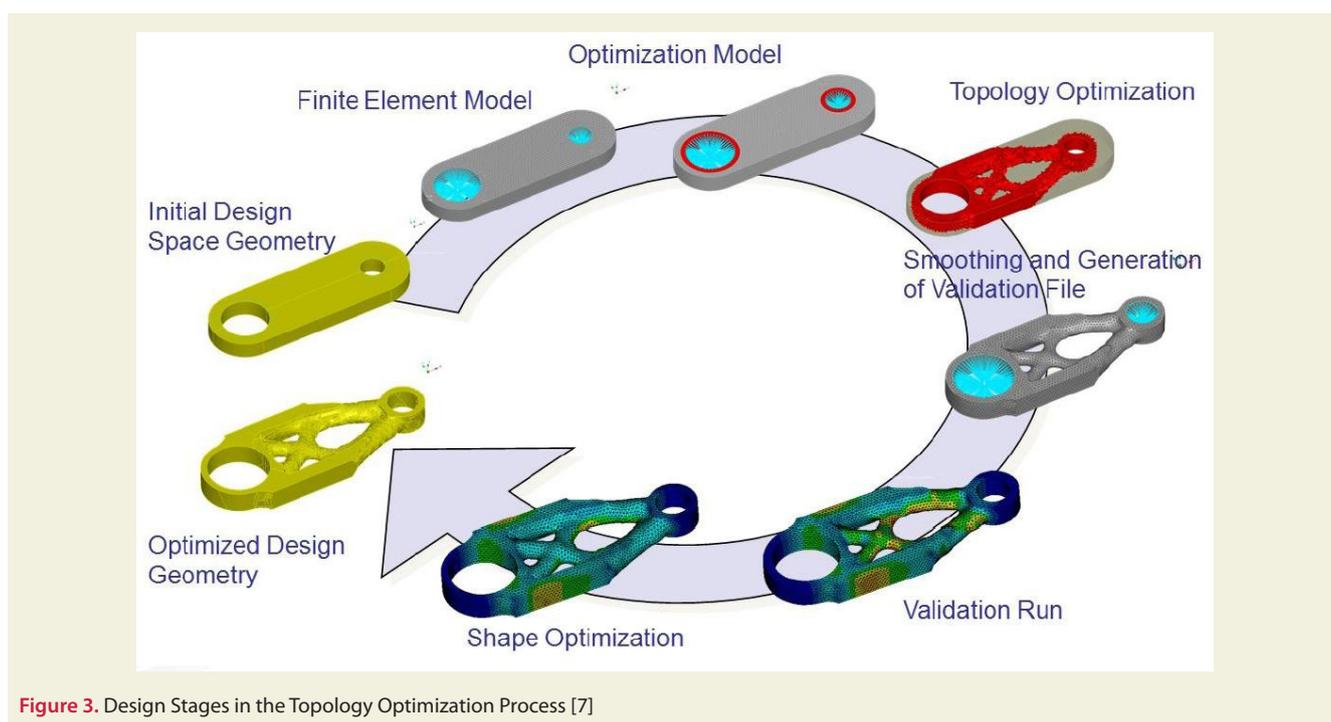
Figure 3. Design Stages in the Topology Optimization Process [7]
