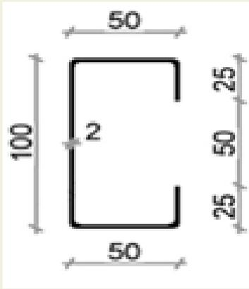
Figure 17. Dimensions of Dip Galvanised Steel with C Profile Structure [22]
