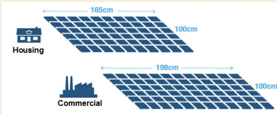
**Figure 15.** Dimensions of solar Panel Used in residential and commercial areas [21].
