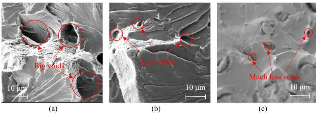
Figure 5. Scanning electron microscope views according to infill ratios of Concentric filling pattern, a) 20%, b.) 60%, c) 95%.
