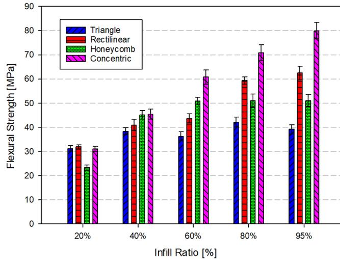
Figure 3. The flexural test properties of the samples.
