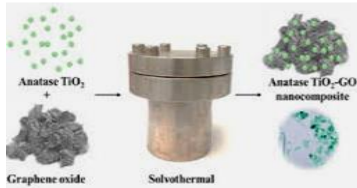
Figure 9: Synthesis of Nanoparticle using Solvothermal Method (24).
