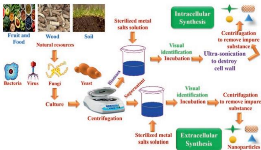
Figure 6: Green synthesis of nanoparticles by various microorganisms (168).
