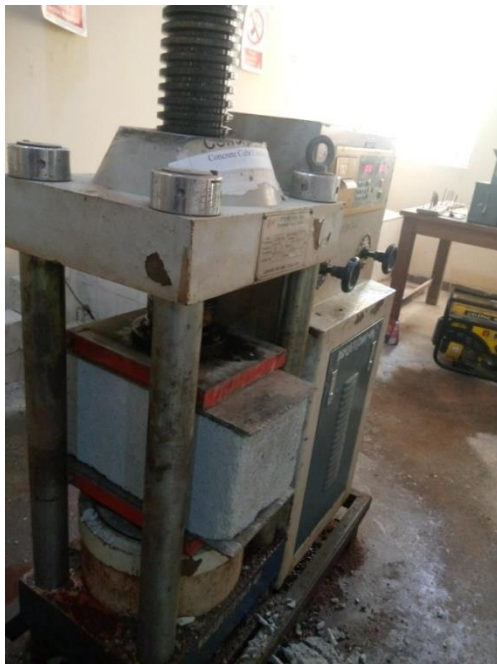
Figure 3. Sandcrete block undergoing compressive strength testing.
