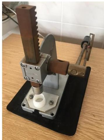
**Figure 1.** Pressing of TD/TMA after impregnation.
