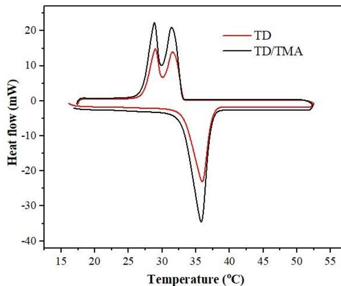
**Figure 4.** DSC thermograms of TD and TD/TMA
