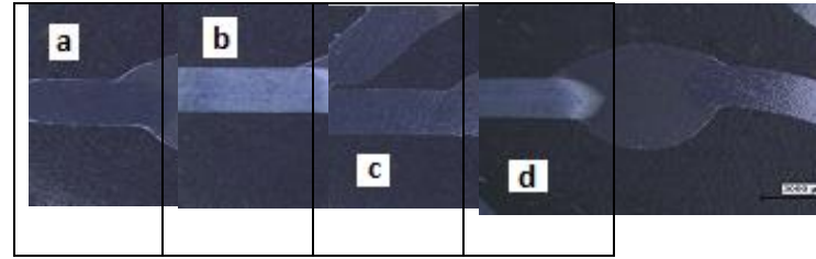
Figure 3. The macro-structure of samples joined by (a) 10 l/min, (b) 12 l/min, (c) 14 l/min and (d) 16 l/min gas flow rate in butt joint form.
