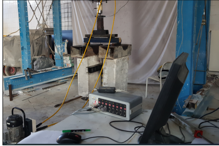
Figure 2. Bending test experimental setup
