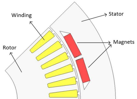
**Figure 4.** Cross-section of the outer-rotor PMaSynRM (Dış rotorlu MD-SRM'nin kesiti)
